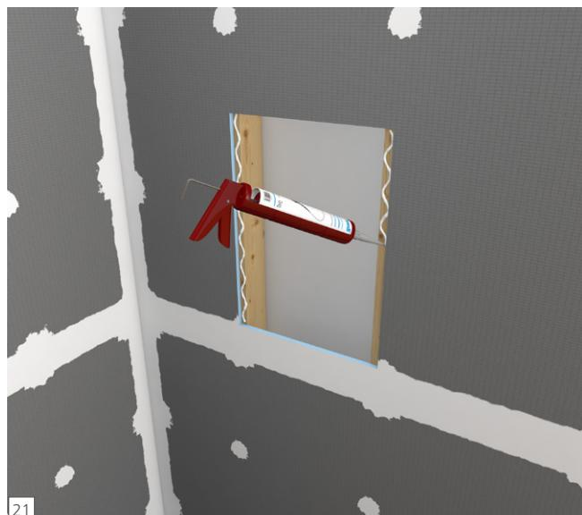
**EN** wedi Niches are installed in a cut out in the wedi wall and attached with it's flange right into the center of 16 in. o.c. studs. wedi Joint Sealant is set along the connection of wall to niche.
