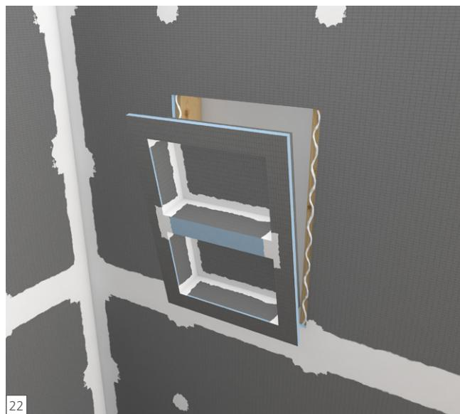
**EN** Fasteners every 12 inches on either side of the niche, or a minimum of 1 fastener on each of the 4 corners, are set to create a flat transition to wall panels. Another 1/2 in. bead of wedi Joint Sealant is spread flat over fasteners and seams.
