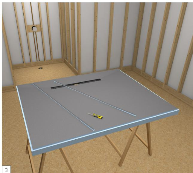
**EN** Once cut, you want to dry fit the base and then remake the 1/2 in. x 1/2 in. perimeter channel where the base connects to wedi Building Panels, curbs, ramps or extensions. Clean the base and channels from saw dust using a vacuum cleaner.
